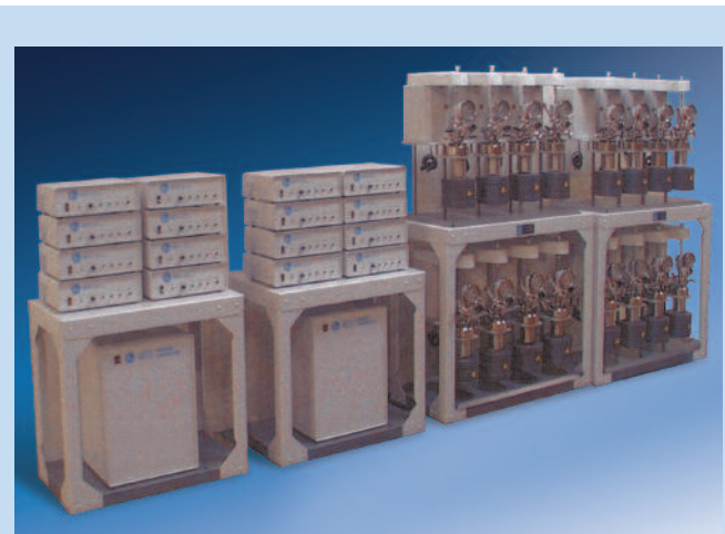
This custom order is set up to run sixteen Reactors, two 4871 Process Controllers, with sixteen 4875 Power Controllers all through one PC.
