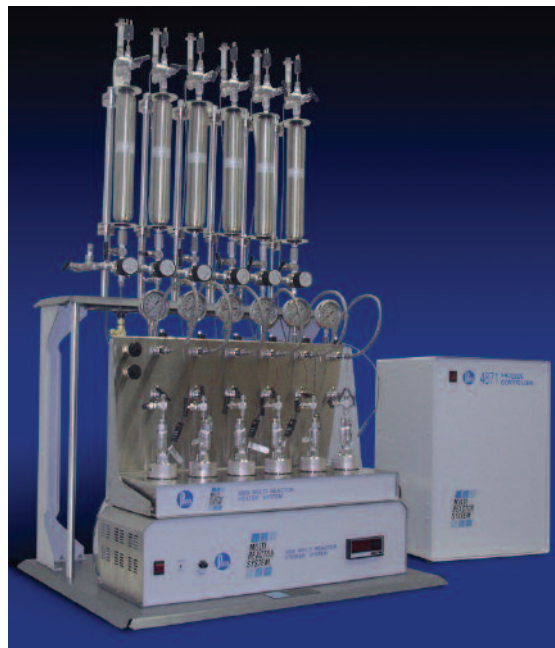
The photo above illustrates a six station multi-reactor system. Each reactor is equipped with its own constant pressure gas delivery system. The 4871 Controller maintains all of the important system parameters, including temperature and stirring speed, and records the gas consumption of each of the reactors.
