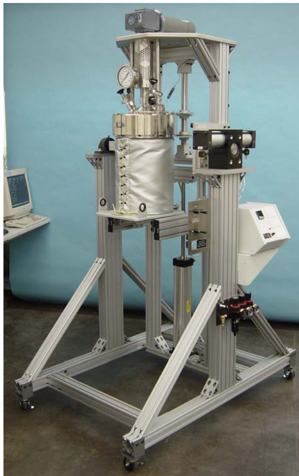
Figure 4 Five gallon reactor in vertical position with pneumatic tilt control.
