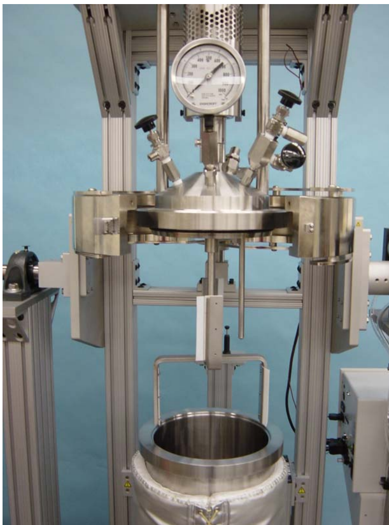
Figure 6 Five gallon internal tumbler stirrer with PTFE wiper blades.
