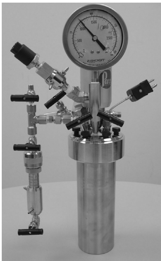
Parr 10 mL Sample Vessel Model 4351-I-D-V-C on 600 mL Mini Reactor
