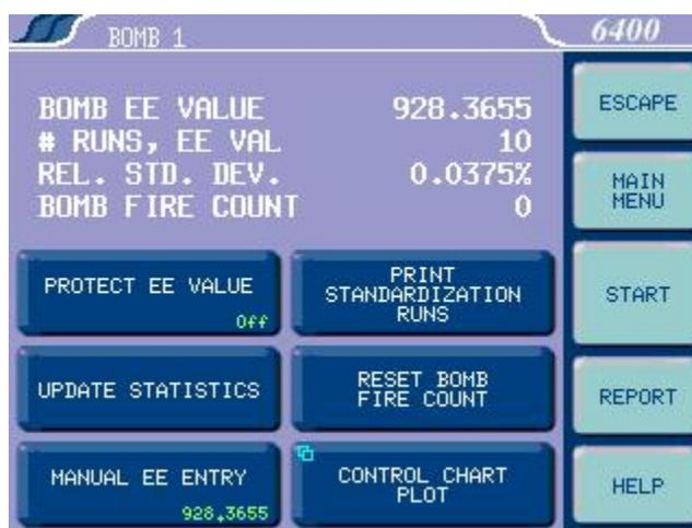
The calibration of any instrument should reflect as closely as practicable, the current state of the measuring system. To this end, the Parr 6000 Series Calorimeters support the calculation
