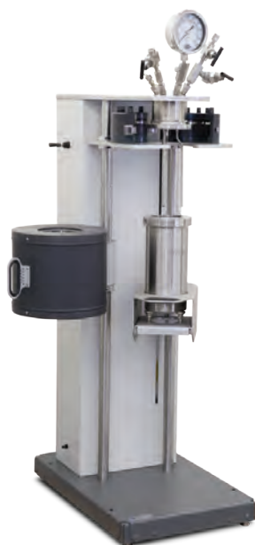
4680-1800mL Fixed Head Vessel shown with Split Rings open and vessel down using a pneumatic lift.
